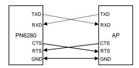
Figure 3-8 Connect to AP method(4lines)
