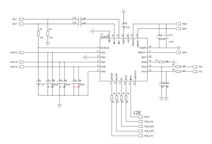
Figure 3-7 NAU8814YG peripheral Circuit (PN6280 as Main device)
