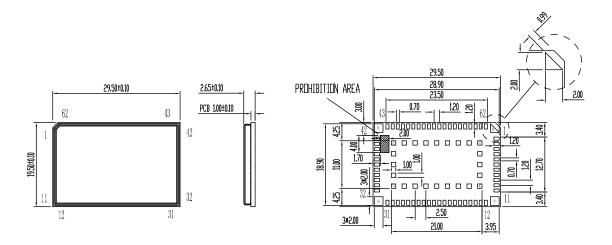
Figure 2-4 Module Size (Unit: mm)
