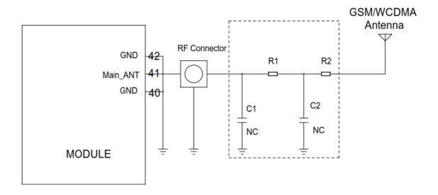
Figure 5-1 Main Antenna Design
