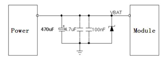
Figure 3-1 Power Supply circuit
