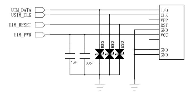
Figure 3-4 (U)SIM Circuit
