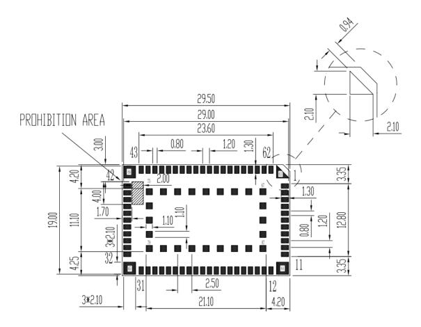
Figure 2-5 Recommend pad (front view, unti: mm)
