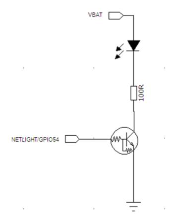
Figure 3-10 LED Circuit
