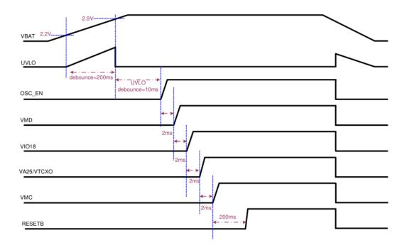
Figure 4-1 Power up time sequence diagram
