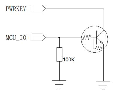
Figure 3-2 Control module boot circuit
